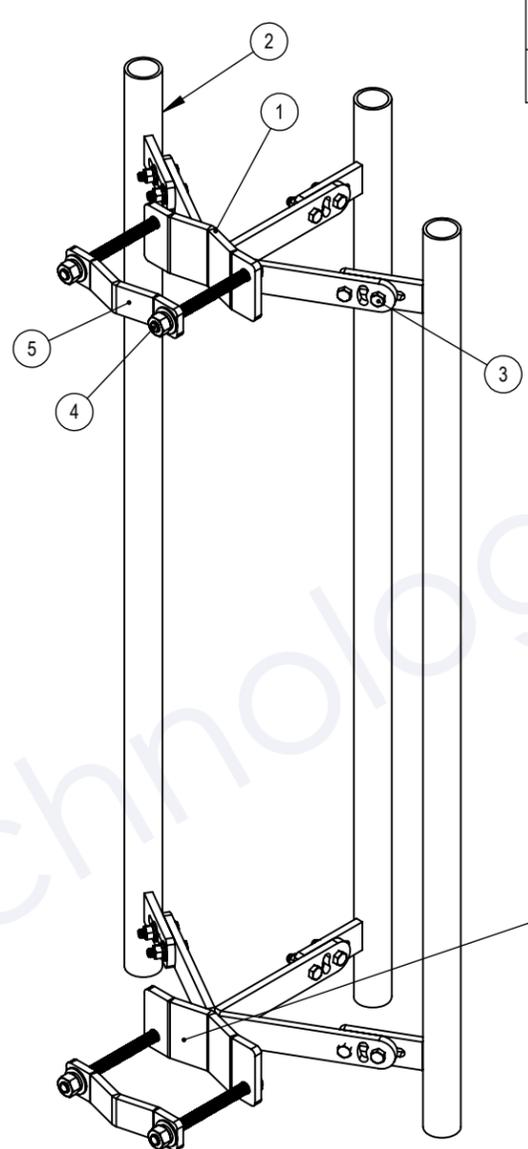
Clamps accomodate 1.25" to 5" pipe and tower leg diameters.
